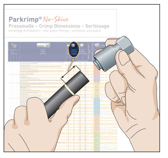
6. Mark the Insertion Depth acc. to the Crimp Dimensions wallchart or www. parker.com/crimpsource-euro and push the hose onto the fitting up to the mark. If necessary, slightly lubricate the nipple end with hydraulic oil.
